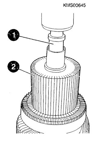
Replacing needle bearing in armature
